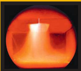
From the thermal image it is clear how strongly the air-gas mix is swirled in the glow zone combustion chamber. This constant movement significantly contributes to a low-residue combustion.
